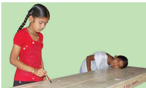
Fig-11: Propagation of sound in solids
