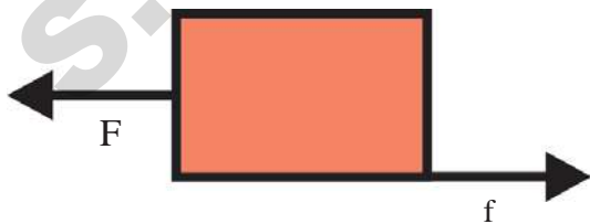
Fig-11: Horizontal forces on the brick
